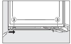
■ Using a flat-headed screwdriver, slide the soft-close mechanism back into the door as far as it will go towards the appliance so that it clicks into position.
